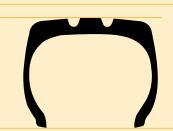
Rock, traction, regular tread 100% of Design Tread Depth E2-E3-L2-L3-G2
